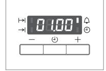
When the time has elapsed, the function indicator flashes and an audible signal sounds for 2 minutes. The signal can be stopped by pressing any button.
